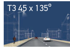
Application: Asymmetric light distribution for Urban road.
