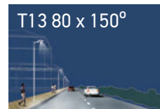
Application: Asymmetric light distribution for Urban road.
